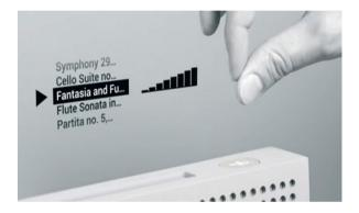
Waves on the radio frequency spectrum are emitted at a target by the chip. The panel then receives the reflected waves, which are transferred to a component that interprets the differences between them. Even subtle change detecting in returning waves can be translated into commands for an electronic device.
